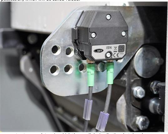
Tcloud will guarantee to granulators in which the small device (in the photo) and some sensors will be installed, to be connected to the cloud. Thanks to these sensors that will transmit the data to the cloud and the web platform developed together with CombiQ, it will be possible to monitor all the operating parameters of the granulator in real time, extrapolate the data and analyze them, scheduling ordinary maintenance interventions in advance.
