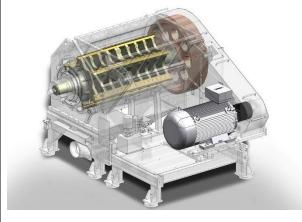
The rotation of the rotor does not produce the very detrimental "drag" effect, meaning the mass of material being ground in the cutting chamber does not rotate with the rotor producing lots of dust and fine particles, that will all become waste through the washing line. The production of fine particles is reduced to few percentage points, versus a common 15% or more from conventional granulators. The rotor is of open type design, taking only 30% of the cutting chamber volume.
