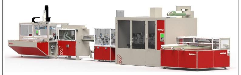
The Povi 5000 and Povi 10000 models for off-line punching can reach speeds of up to 12 meters per minute. These models are also equipped with an innovative system for handling the conduits inside the various stations of the machine without leaving any visible mark on the bottom of the conduits themselves.
