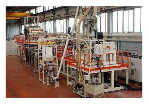
AMUT's technologically advanced solutions, suitable for a wide range of thermoplastic resins, includes extrusion lines for sheets, plates and multicellular panels with nominal widths from 400 to 3,300 mm and thicknesses from 150 microns to a few centimeters. The number of co-extruders is defined according to the specific needs of the processor and to the features of the finished product.
