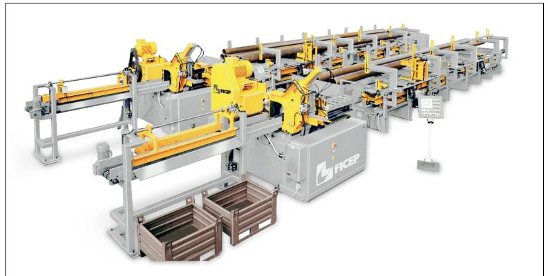
**The VS Series** high-speed saws are characterized by the blade operating vertically from bottom to top. This series is particularly suitable for cutting plates, pipes and shaped profiles, utilizing the full stroke of the bottom blade. In addition to offering versatility in cutting various types of profiles, the VS Series sawing machines have the advantage of a free worktable, facilitating the introduction of material and allowing rapid blade changes.
