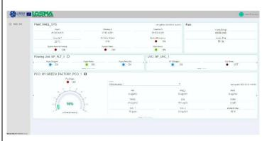
The plant's dashboard displays the data collected by the IoT Air Quality Monitor sensors to allow users to monitor air pollutant parameters at all times. From PM₁-100 to VOCs and CO₂ values in the air, this software is used as a process management panel, providing an overall view of the plant's air quality.
