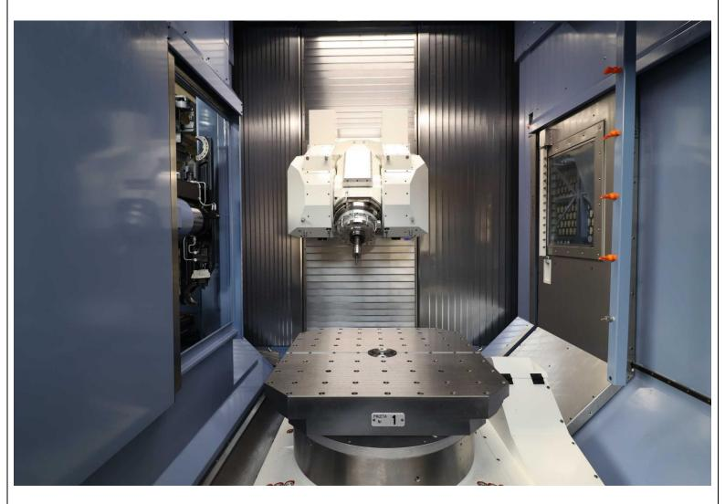
The high machining precision obtained with the Tank 1900, a medium-large machine with considerable structural rigidity, is the result of great attention to all construction aspects, to the geometric precision of the machine, to the thermo-mechanical symmetry and to the excellent components used.
