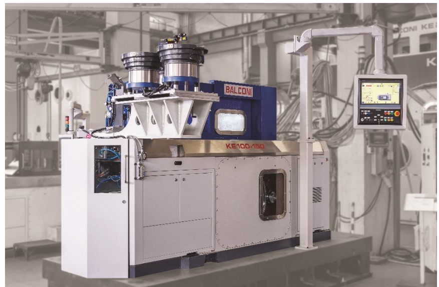
Balconi horizontal extrusion press model KE 100-150 of 1.000 kN and speed up to 330 spm
