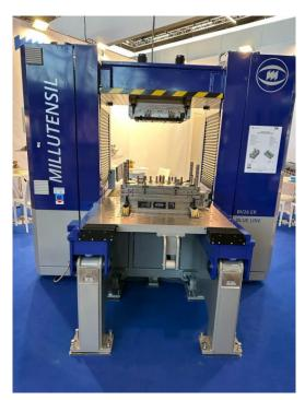
All presses in the series can also be equipped with tilting of the lower platen or table rotation, or a combination of both options, should the customer require it.
