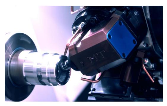
Besides, it is equipped with MTSK Quick Change System, developed by MT, for an accurate and fast replacement of the gear cutter.
