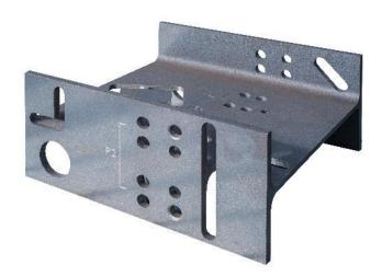
This kind of operations are usually processed with other technologies like oxy-cutting or other machines. Now instead the same can be realized through chip removal with specifically shaped tools and with specific software cycles already integrated in the machine.
