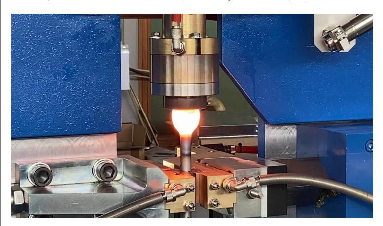
It has been found that this combination of the AC Inverter and brushless motors to be the best solution due to the extreme precision in controlling each stage of the production of the bulb shapes and suitable for meeting tight tolerances making easier and more precise the final forging on a DD Press.
