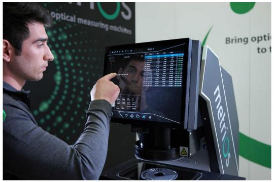
But here's the solution: the Metrios on-board step master and 3 temperature sensors monitor the thermal deformations of the machine. There is no need to locate the machine in a metrology lab - it has been designed to stay in production.
