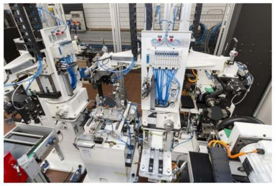
Balancing system for electric rotors consisting of two stations, one for unbalance measurement on two planes with belt drive and one unbalance correction station for axial drilling on the sides through two opposed units with controlled axes.
