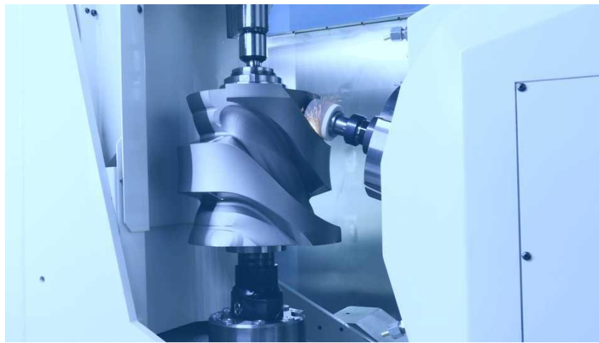
Cam grinding operations on TANK 1300 Multitasking with wheel dressing on board
