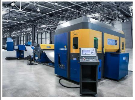
So, in order to maximize production, making it faster and completely automated, Produtech specialized in designing, implementing and marketing systems for processing metal coils through laser cutting and/or punching-forming technologies.
