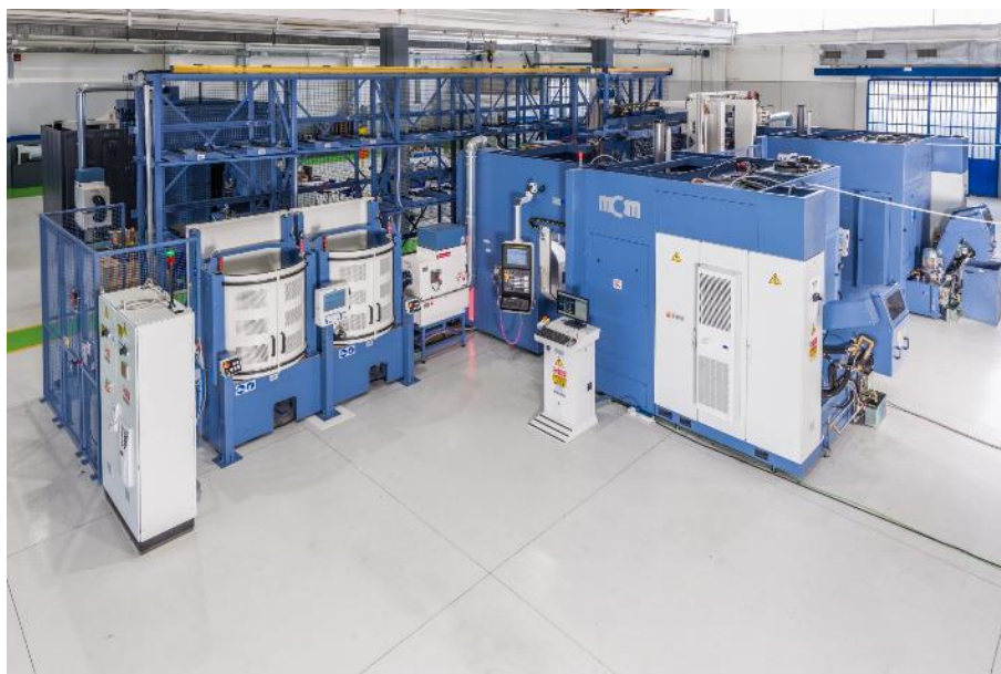
MCM FMS _ 2 operator's places for parts loading unloading and jFMX supervision software
