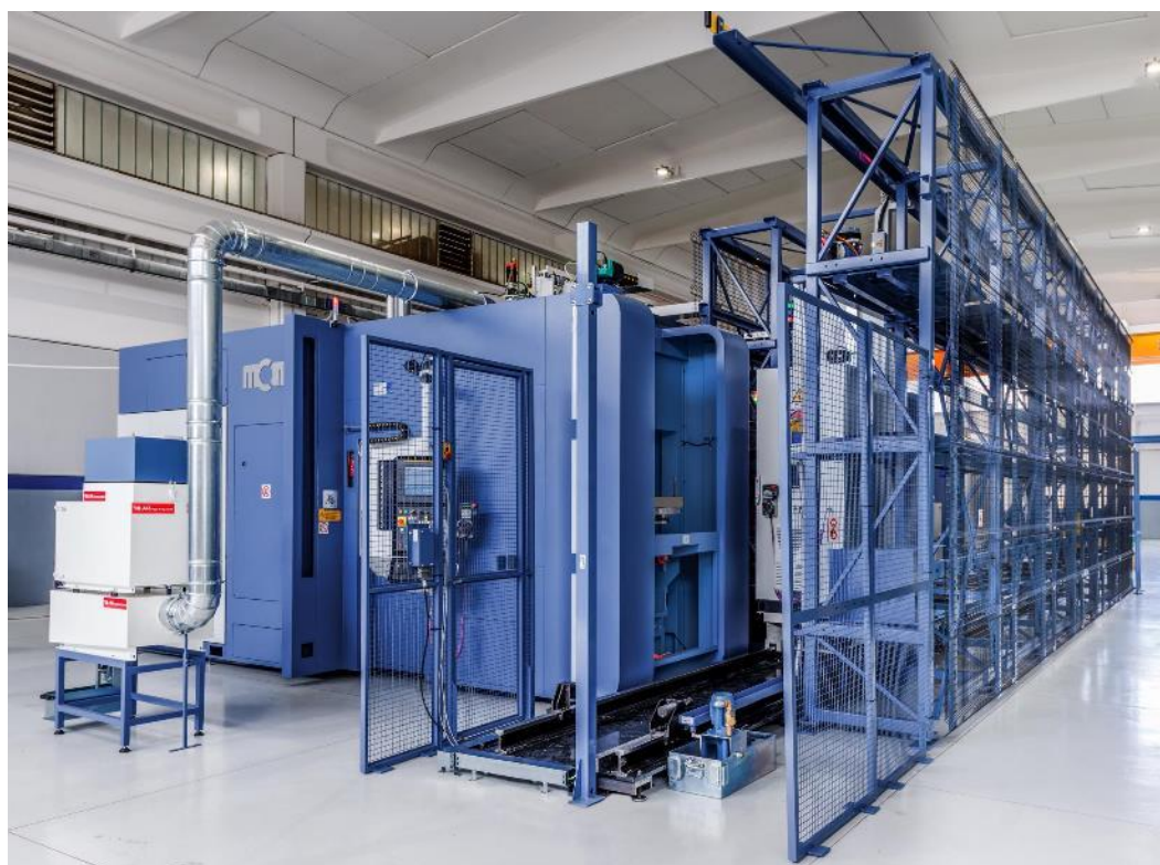
MCM FMS_ 42 pallet storage places on 3 levels
