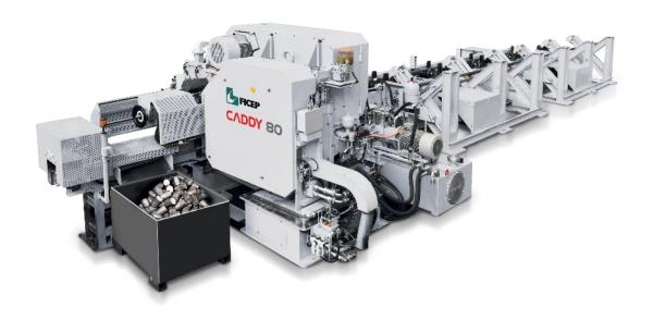
CADDY range of mechanical horizontal slide shears can cut any type of material and, within the forging and stamping production cycle, is placed at the head of the process bringing a high contribution in terms of efficiency in the most varied fields of application, meeting the needs of:
