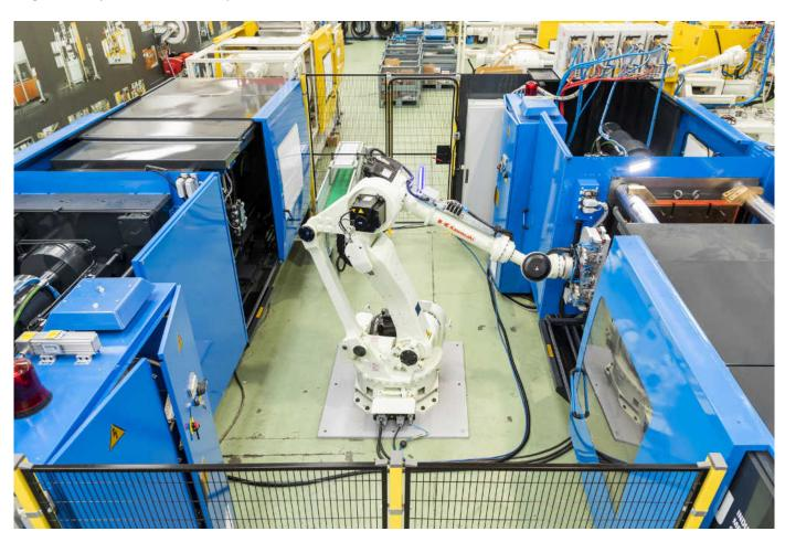
The company supplies robotised cells based on the 14 models of injection moulding machines in its portfolio, making them communicate with each other, and equipping them with accessories such as anthropomorphic robots or conveyor belts.
