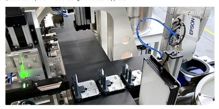
The magnetic shuttles float seamlessly on the pathways with a fast and fluid motion, reaching a speed of 2 m/s, with an impressive acceleration and deceleration. GEFIT is also constantly focused on taking full advantage of the opportunities of the magnetic levitation platform, streamlining processes, and optimizing dimensions to obtain more compact and efficient machines.
