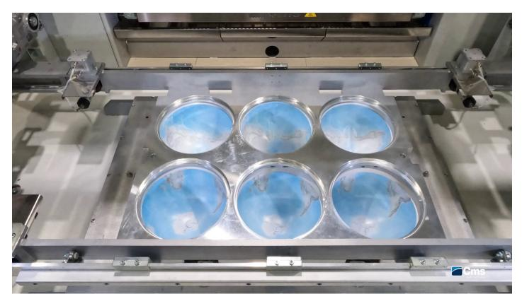
The fully automatic management of the process ensures high stability and repeatability of material stretching and shaping operations, as a result obtaining high and consistent quality in every production cycle. For this particular product, the machine is equipped with a six-cavity mould for 0.6 mm thick silk-screen printed polypropylene sheet and an alignment system with an accuracy of ±0.2 mm, which guarantees uniform results on each piece.
