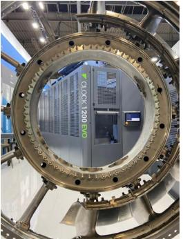
maximum grinding disc diameter of 300 mm, revived by a driven disc placed within the workarea. The grinding disc wear is accurately assessed and compensated by a four-step process that guarantees that the sizes of the final piece are maintained. This process involves the pre-grinding of the piece on the disc, measuring the size obtained with the probe, subsequent correction of the depth of cut if required and finally finishing. All steps are supervised by a software.
