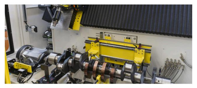
Our ZBK200 machine is specifically designed to automatically achieve all the required tasks for the balancing of crankshafts up to a maximum weight of 200 kgs.
