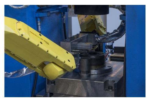
The Direct Drive presses from Ficep allow for precise control of speed, energy, and generated force. By integrating 6-axes and 4-axes robots from the RF and RP series, respectively, direct control over critical factors such as temperature and lubrication is achieved. The high performance delivered by these presses, combined with total control over the production cycle, makes Ficep offering particularly valued in sectors with stringent production parameters.
