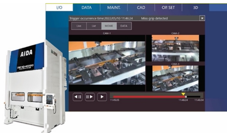
* The Drive Recorder starts automatically and enable viewing of the in-die footage when a fault occurs.
