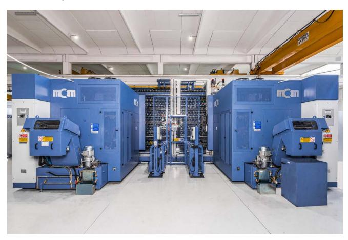
Therefore the presence of two identical tools in both magazines, serving the relevant machines, is no longer required, but one tool in the shared magazine is sufficient to meet the needs of both machines.
