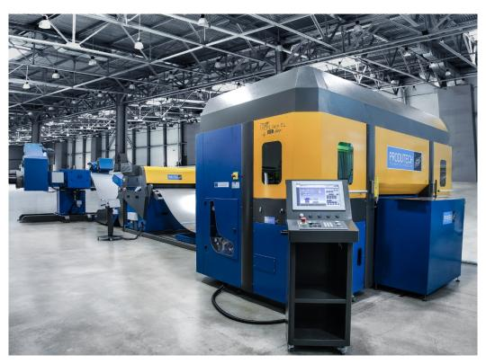
Also, the processed parts can be marked with logos, and it is possible to make deep-drawing, air vents, ribs (even curvilinear, by means of suitable wheel-tools), small beads and references for folds. All the processes - including cutting - are made with mechanical tools that do not produce fumes or incandescent scraps, so they do not affect superficial finishing or any potential protective films on the processed materials.
