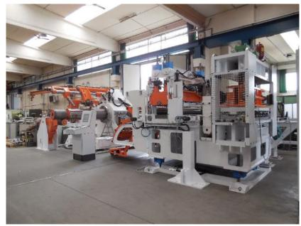
In a context in which the market trend sees a continuous increase in the use of always wider sheet metal formats and coils with increasingly greater capacity, the company responds with products that adapt well to these needs. The company is able to realize lines with decoilers with a capacity up to 30 t, with an external diameter up to 2,000 mm, with strip widths up to 2,000 mm, for thicknesses up to 18 mm .
