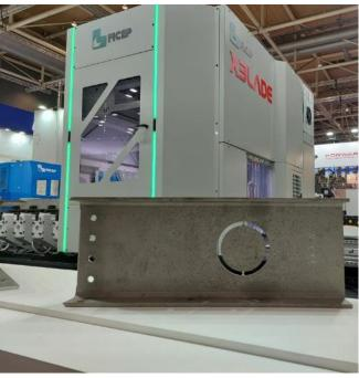
The innovative feature of XBLADE is the ability to perform three-axis processing even on inclined planes, in two different directions. The 5-axis head consisting of two rotating wrists allows the tool to be positioned at virtually any point in the working space. The working area is delimited with light barriers. It is a moving column machine in which the longitudinal X-axis can be configured on request with one-meter pitch.
