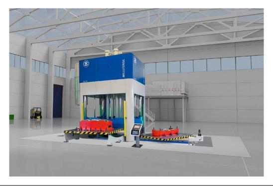
Spotting presses belonging to the BV-Series not only are used for the assembly, adjustment, inspection and repair of small-sized moulds, but also for splitting, setting, maintenance and trial operations. The presses are suitable for tools and moulds made of thermoplastics, die casting, thermosetting plastics, rubber and punching.
